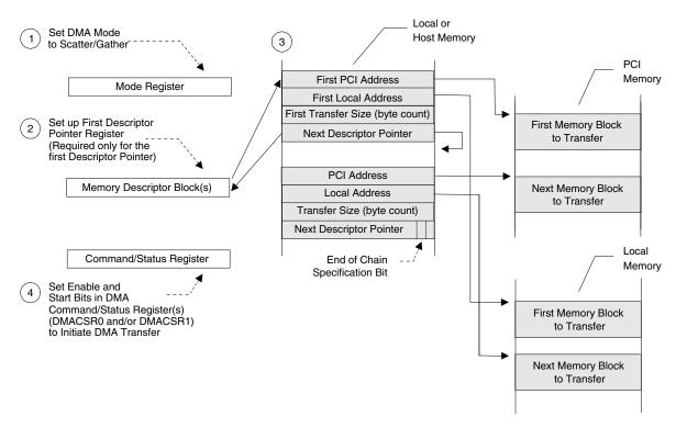
Figure 3-17. Scatter/Gather DMA Mode Descriptor Initialization [PCI SAC/DAC PCI Address (DMADAC0 and/or DMADAC1) Register Dependent]
