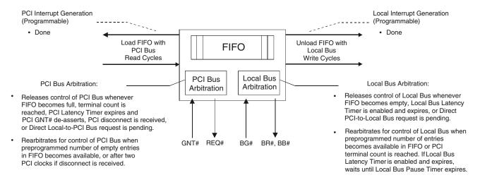
Figure 3-20. PCI-to-Local Bus DMA Data Transfer Operation
