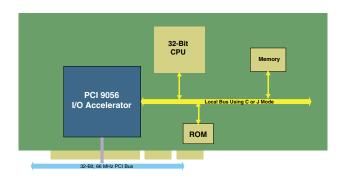
Figure 1-5. PCI 9056 PC Adapter Card with C or J Mode Processor
