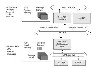
Figure 7-1. Typical I<sub>2</sub>O Server/Adapter Card Design
