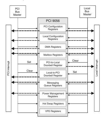
Figure 2-6. PCI 9056 Internal Register Access
