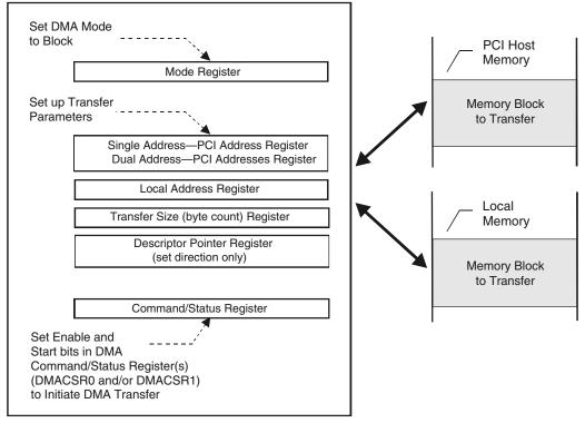
Figure 5-11. Block DMA Mode Initialization (Single Address or Dual Address PCI)
