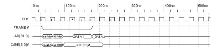
Figure 3-5. Dual Address Timing
