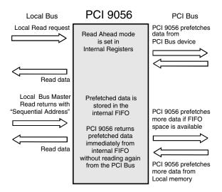
Figure 3-4. Direct Master Read Ahead Mode
