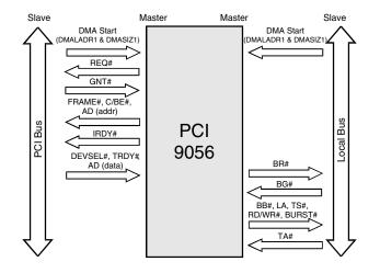
Figure 3-12. DMA, PCI-to-Local Bus
