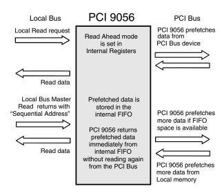
Figure 5-4. Direct Master Read Ahead Mode
