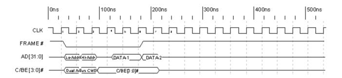
Figure 3-14. Dual Address Timing
