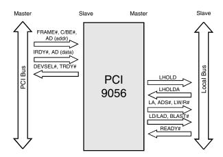
Figure 5-8. Direct Slave Write
