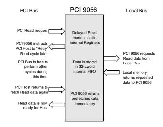
Figure 5-6. Direct Slave Delayed Read
