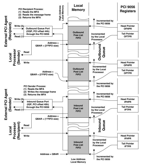
Figure 7-3. I<sub>2</sub>O Circular FIFO Operation
