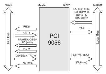
Figure 3-2. Direct Master Write
