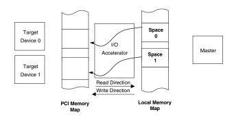
Figure 1-1. Direct Master Address Mapping
