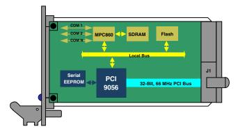
Figure 1-4. PCI 9056 CompactPCI Peripheral Card
