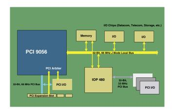
Figure 1-9. PCI 9056 Embedded Host System with IOP 480
