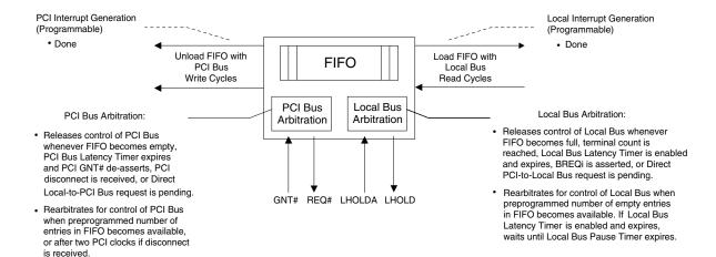
Figure 5-19. Local-to-PCI Bus DMA Data Transfer Operation
