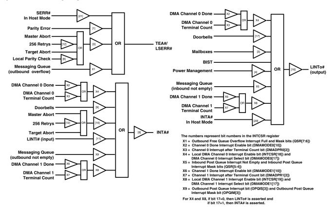
Figure 6-1. Interrupt and Error Sources
