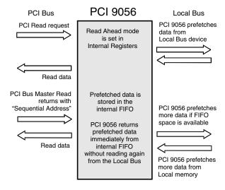
Figure 3-7. Direct Slave Read Ahead Mode
