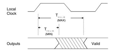
Figure 13-2. PCI 9056 Local Output Delay
