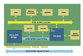
Figure 1-6. PCI 9056 PC Adapter Card with Local PCI I/O and PCI-to-PCI Bridge
