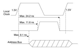
Figure 13-3. PCI 9056 ALE Output Delay to the Local Clock at 33 MHz Clock
