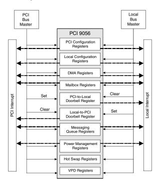
Figure 4-6. PCI 9056 Internal Register Access
