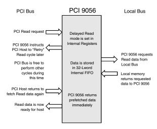
Figure 3-6. Direct Slave Delayed Read
