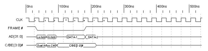
Figure 5-5. Dual Address Timing
