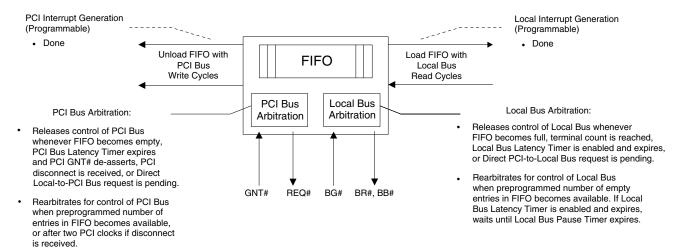
Figure 3-19. Local-to-PCI Bus DMA Data Transfer Operation
