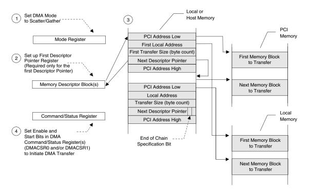
Figure 5-18. Scatter/Gather DMA Mode Descriptor Initialization [DAC PCI Address (DMAMODE0[18] and/or DMAMODE1[18]) Descriptor Dependent] (PCI Address High Added)
