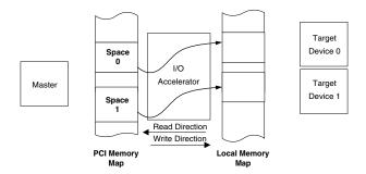
Figure 1-2. Direct Slave Address Mapping
