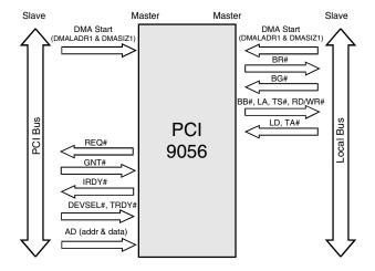
Figure 3-13. DMA, Local-to-PCI Bus
