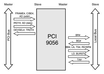
Figure 3-8. Direct Slave Write
