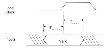
Figure 13-1. PCI 9056 Local Input Setup and Hold Waveform
