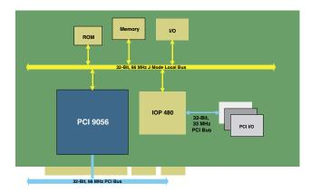
Figure 1-7. PCI 9056 PC Adapter Card with Local PCI I/O and IOP 480
