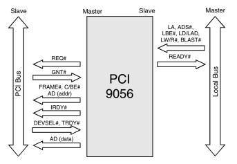
Figure 5-2. Direct Master Write
