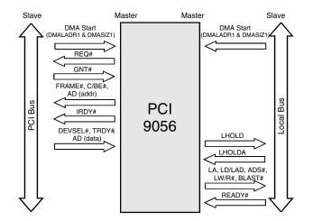
Figure 5-12. DMA, PCI-to-Local Bus
