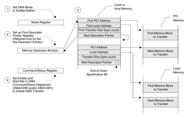
Figure 5-17. Scatter/Gather DMA Mode Descriptor Initialization [PCI SAC/DAC PCI Address (DMADAC0 and/or DMADAC1) Register Dependent]
