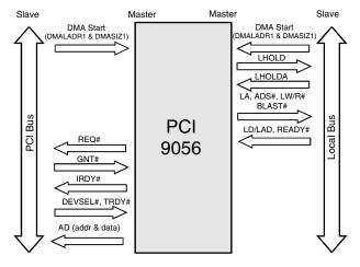
Figure 5-13. DMA, Local-to-PCI Bus
