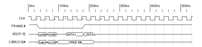
Figure 5-14. Dual Address Timing
