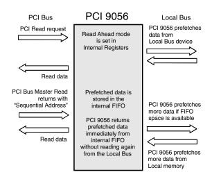
Figure 5-7. Direct Slave Read Ahead Mode
